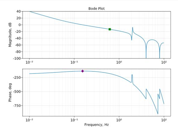
The Bode plot shows magnitude and phase vs. frequency. The gain margin may be read from
