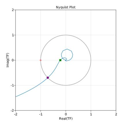
The Nyquist plot is just the transfer function itself plotted in the complex plane. The gain and phase margins may be deduced from where the transfer function crosses the unit circle, and where
