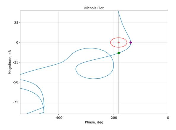
The Nichols plot is magnitude vs. phase. The gain and phase margins are the same as in the Bode
